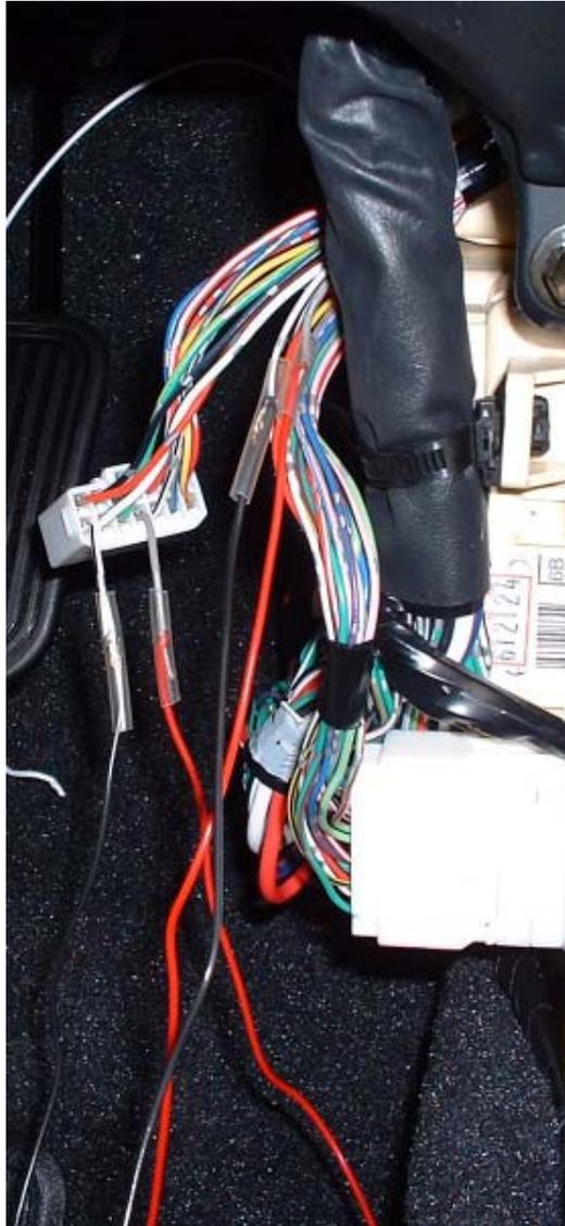
Put the wires into a sheath or use insulation tape to protect them. Make sure you don't get them mixed up! You need to be able to identify which pair comes from the connector and which ones go to the mirrors. **THIS IS VERY IMPORTANT!**
