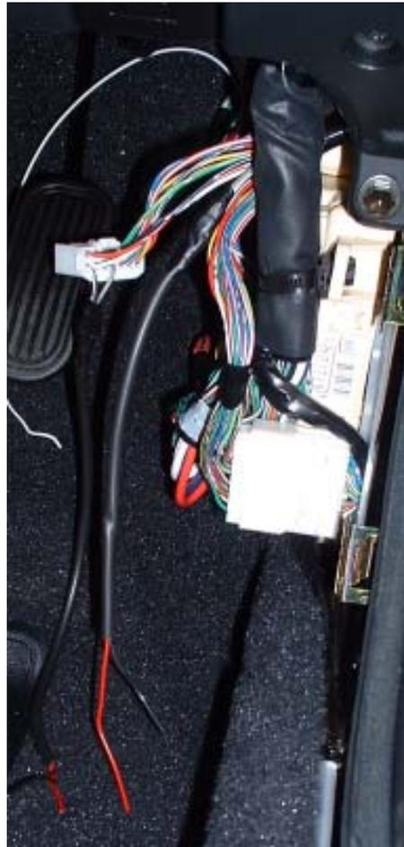
Now locate the alarm trigger wire. This is in the lower right connector, coloured green. Do NOT CUT this wire. Simply bear it's sheathing and connect to it. You can also use a scotchblock for this.
