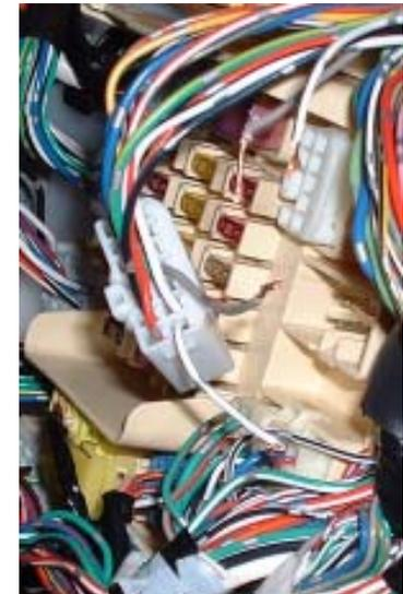
Now extend these wires. It will be hard to get cable of the same colour, so use black and red to identify the polarity easily. I prefer to use heat shrink tubing instead of insulation tape.
