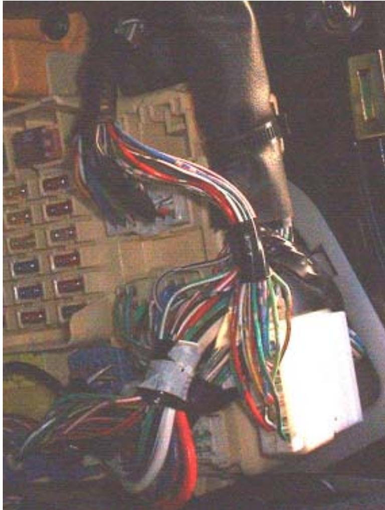
Select a permanent Positive and earth for the power. I already had one for my mobile phone taken from the ignition but there are a few there that can supply ample power. If you are testing for a permanent live around the ignition area, DO NOT touch the yellow wire. This is for the airbag and can trigger it.
