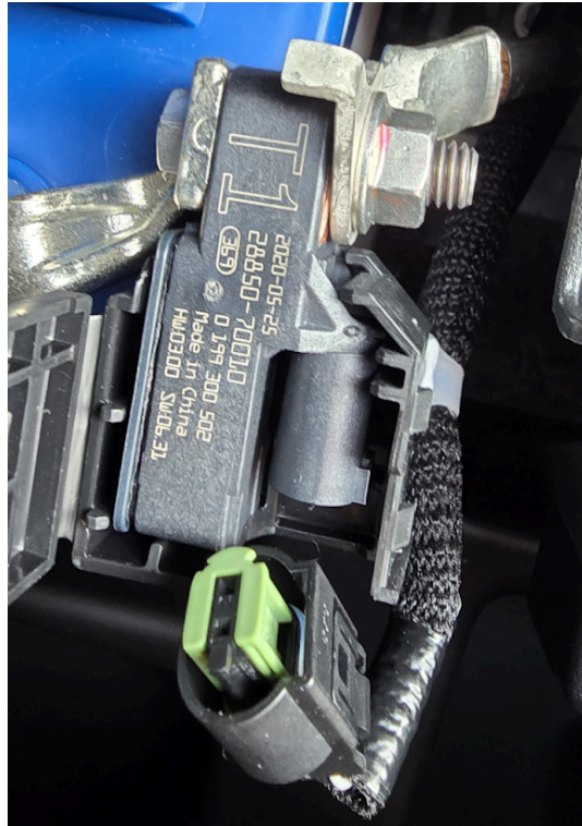
The 12v battery negative terminal sensor plug
